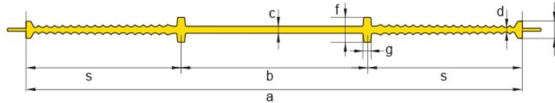
They are the type of waterstop gaskets placed inside the concrete construction element used in joints for raft – raft foundation, raft foundation -retaining wall, retaining wall - retaining wall joints. They are produced in three different widths (240, 320, 500 mm).
